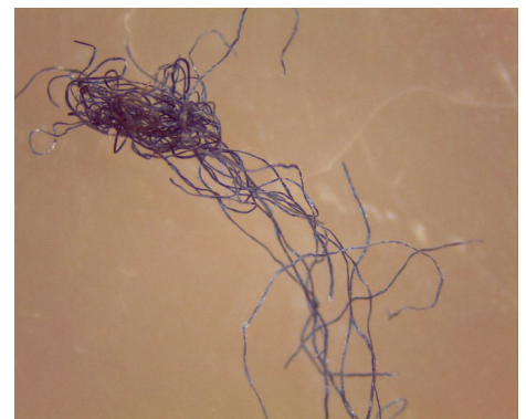
Plastic fragments, films, beads, and fibers within 1 mm of a microscope's viewing area (left). Microscopic fibers (center and right) from synthetic clothing are the most common form of microplastic pollution. The fibers can form tight balls in the gut tract of small animals that ingest them.
