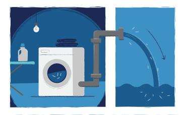
Wash cycle shakes loose thousands of fibers too small to be filtered out by wastewater treatment plants.
